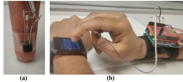
Figure 2: (a) Sensor mounted on finger (b) Hardware Setup
