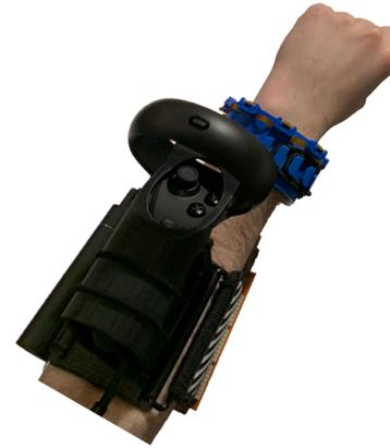
**Figure 11: A Rift-S controller is added to the controller armband to facilitate 6-DoF tracking of the hand.**
